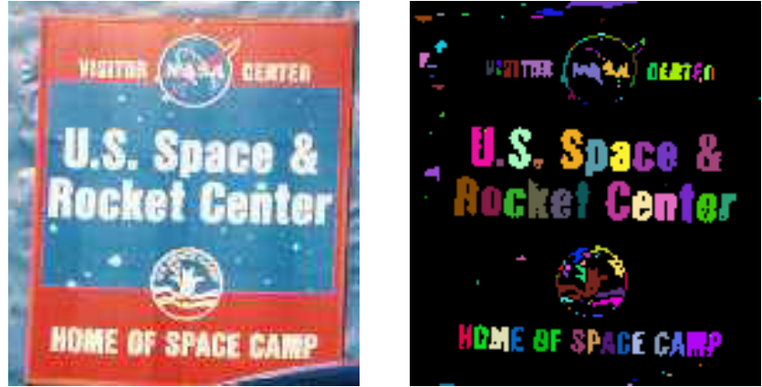
Figure 6.10: “White pixels” are segmented from the color image at the left. Individual connected components of white pixels are arbitrarily labeled by a coloring algorithm as described in Chapter 3. (Analysis contributed by David Moore.)
